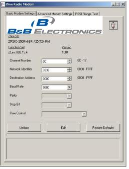
Figure 6. Basic Modem Settings Screen
