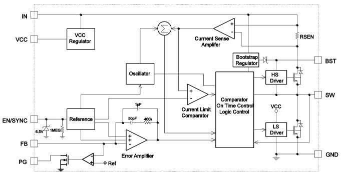
Figure 1: Functional Block Diagram
