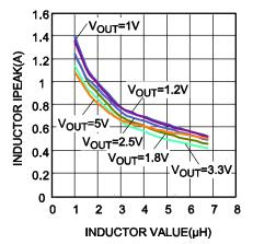
Figure 3: AAM Selection for Common Output Voltages (VIN=4.5V-24V)
