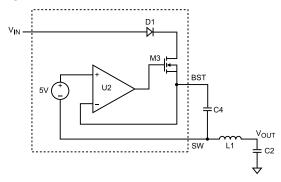
Figure 2—Internal Bootstrap Charging Circuit
