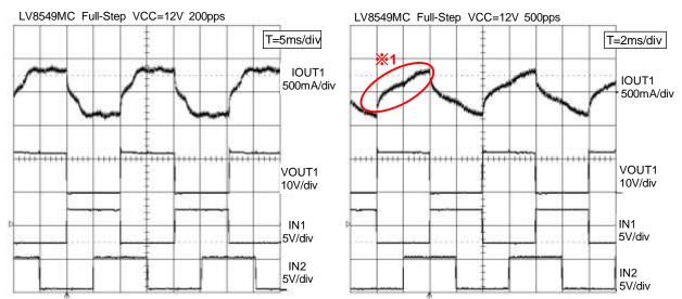
\*1. When the motor rotation is at a high speed, current gradient increases by the inductance of motor (L).
