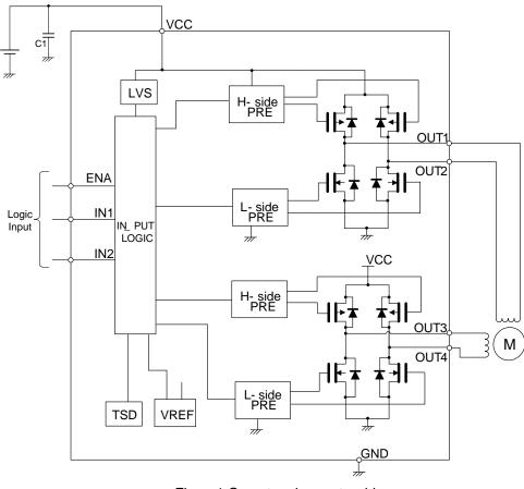
Figure1 One stepping motor drive
