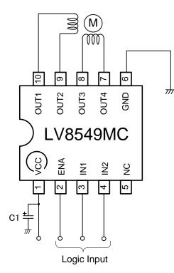
\* Bypass capacitor (C1) connected between V<sub>CC</sub>-GND of all examples of applied circuit recommends the electric field capacitor of  $0.1\mu$ A to  $10\mu$ A.
