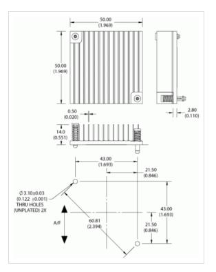
Width: 50.00 Length: 50.00 Height: 14.00 Base Thickness: 2.80 Fin Thickness: Length , Width 0.50 # of Fins: Length , Width 14 Fin Tip to Tip: Finish: AavSHIELD 3C
