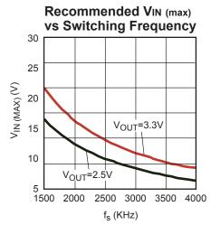
Figure 2—Recommend Max V<sub>IN</sub> vs. f<sub>s</sub>
