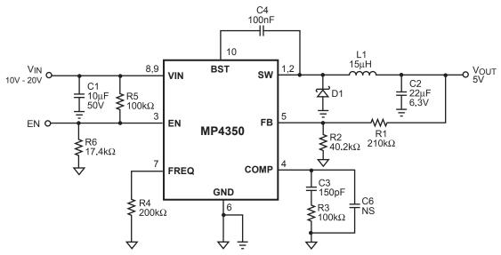
Figure 5—5V Output Typical Application Schematic
