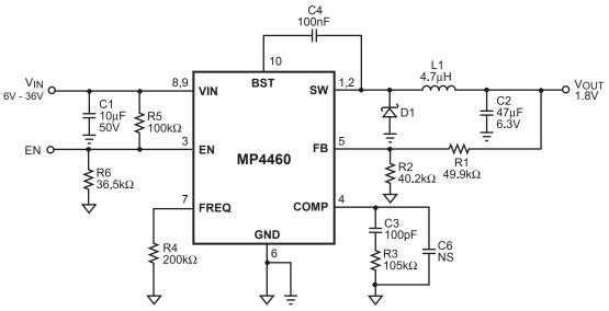
Figure 4—1.8V Output Typical Application Schematic
