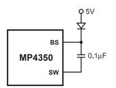
Figure 3—External Bootstrap Diode
