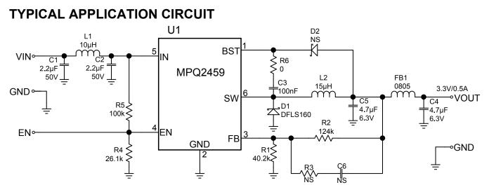
Figure 4: Typical Application Circuit with EMI Concern
