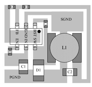
Figure 2: PCB Layout
