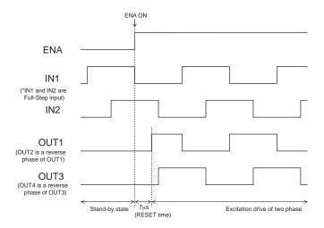
3. Example of current waveform at full-step mode.
