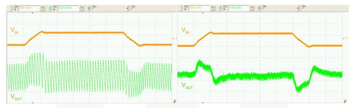
Figure 20. Line Transient 3.3  $V_{IN}$  to 3.9  $V_{IN}$ , 50 mA Load, 10  $\mu$ s/div.
