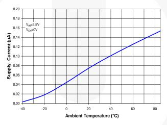
Figure 19. Shutdown Current vs. Temperature
