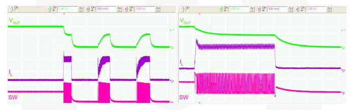
Figure 35. Over-Current Fault Response,  $R_{LOAD}$  = 1  $\Omega$ , 50  $\mu$ s/div.
