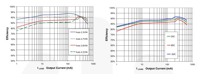
Figure 5. Efficiency vs. Load Current and Input Supply Figure 6. Efficiency vs. Load Current and Temperature
