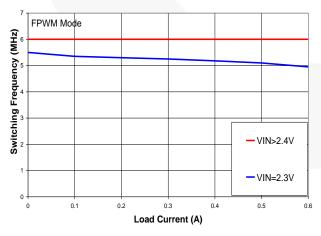
Figure 14. Effect of t<sub>OFF(MIN)</sub> on Reducing Switching Frequency
