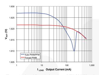
Figure 11. Load Regulation, Auto PFM / PWM and Forced PWM
