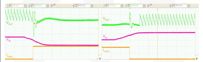
Figure 22. Combined Line/Load Transient 3.9 to Figure 23. Combined Line/Load Transient 3.3 to 3.9  $V_{\text{IN}}$  3.3  $V_{\text{IN}}$  Combined with 40 mA to 400 mA Load Transient Combined with 400 mA to 40 mA Load Transient
