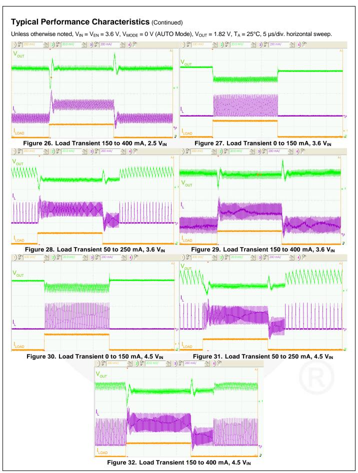
Unless otherwise noted,  $V_{IN} = V_{EN} = 3.6 \text{ V}$ ,  $V_{MODE} = 0 \text{ V}$  (AUTO Mode),  $V_{OUT} = 1.82 \text{ V}$ ,  $T_A = 25^{\circ}\text{C}$ , 5  $\mu\text{s/div}$ . horizontal sweep.
