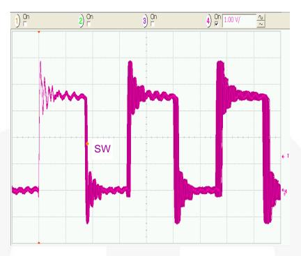
Figure 39. SW-Node Jitter (Infinite Persistence), I<sub>LOAD</sub> = 200 mA, 50 ns/div.
