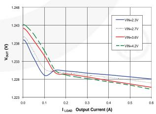
Figure 10. 1.233 V<sub>OUT</sub> Load Regulation vs. Input Supply
