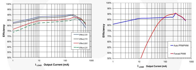
Figure 7. 1.233 V<sub>OUT</sub> Efficiency vs. Load Current and Supply
