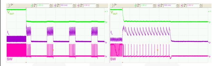
Figure 33. Metallic Short Applied at  $V_{\text{OUT}}$ , 50  $\mu \text{s/div}$ .
