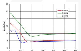
Figure 12. 1.82 V<sub>OUT</sub> Peak-to-Peak Output Voltage Ripple
