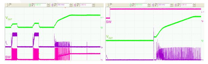
Figure 37. Overload Recovery to Light Load, 50 µs/div.
