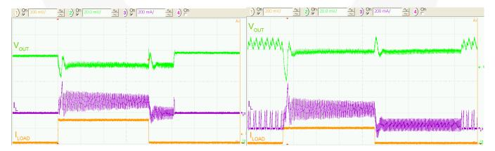
Figure 24. Load Transient 0 to 150 mA, 2.5 VIN
