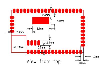
Figure 10: WF121-A recommended PCB land pattern
