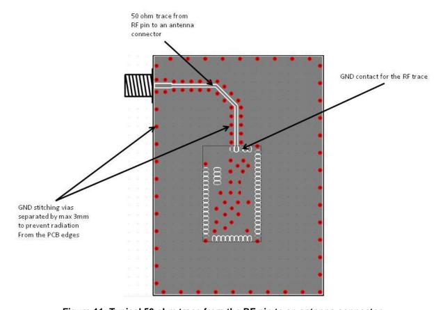
Figure 11: Typical 50 ohm trace from the RF pin to an antenna connector
