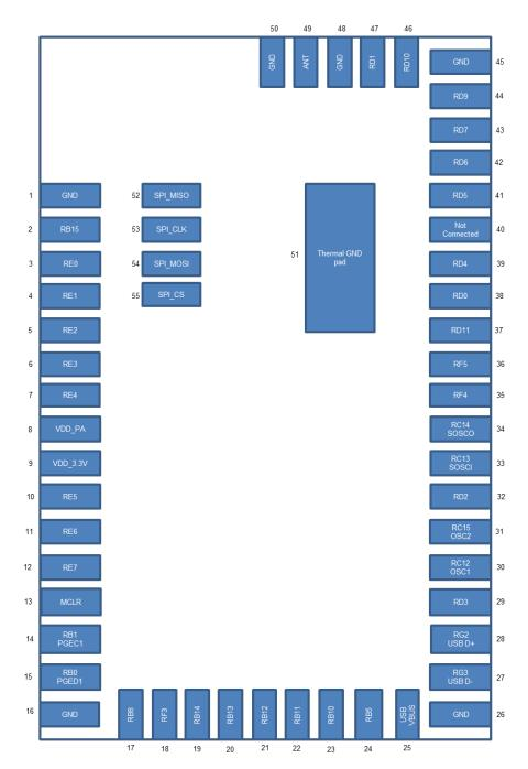
Figure 1: WF121 pinout
