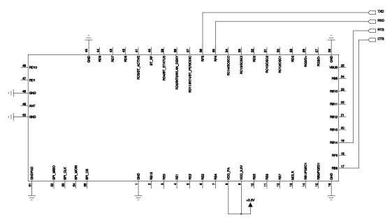
Figure 6: Minimal system required for UART host connection
