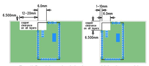
Figure 13: Example layouts, board edge placement on left, board corner on right
