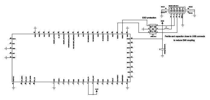
Figure 7: Recommended connections as a USB device. If permanently connected to a hub on the same board, the ESD protection and ferrite can be left out and VUSB can be permanently tied to a supply voltage
