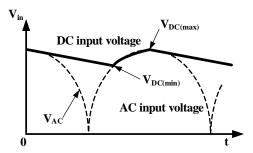
Figure 6: Input voltage waveform
