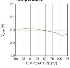
Under Voltage Protection Reference vs. Junction Temperature
