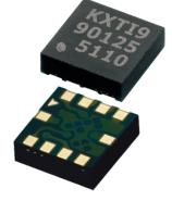
The KXTI9 has internal voltage regulators that allow operation from 1.8 V to 3.6 V and is delivered in a 3x3x0.9mm, 10-pin, LGA package with an operating temperature range of -40°C to +85°C.
