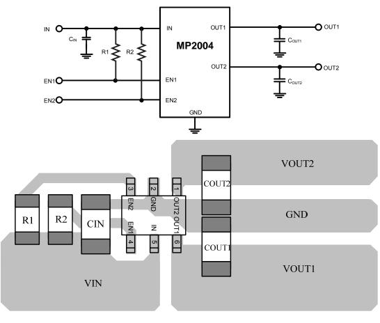
Top Layer Figure 5—PCB Layout
