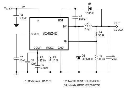
Figure 10. 1MHz 5V to 3.3V/2A Step-down Converter
