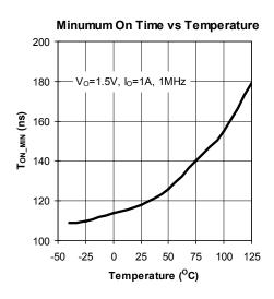
Figure 4. Variation of Minimum On Time with Ambient Temperature
