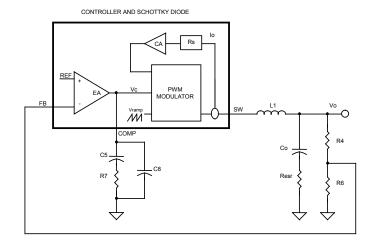
Figure 7 — Block diagram of control loops
