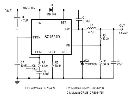
Figure 11. 500kHz 10V-16V to 1.5V/2A Step-down Converter
