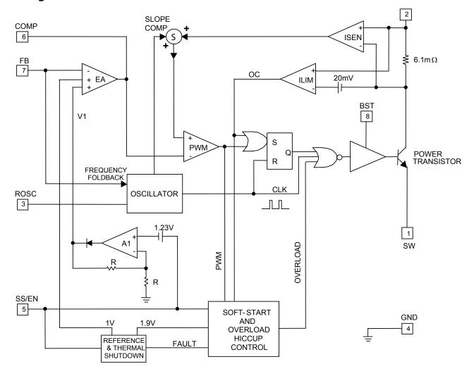
Figure 2. SC4524D Block Diagram
