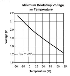
Figure 5 — Typical Minimum Bootstrap Voltage required to Saturate Transistor (I<sub>sw</sub>= -2.6A).
