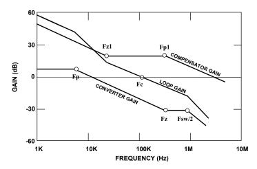
Figure 8 — Bode plots for voltage loop design
